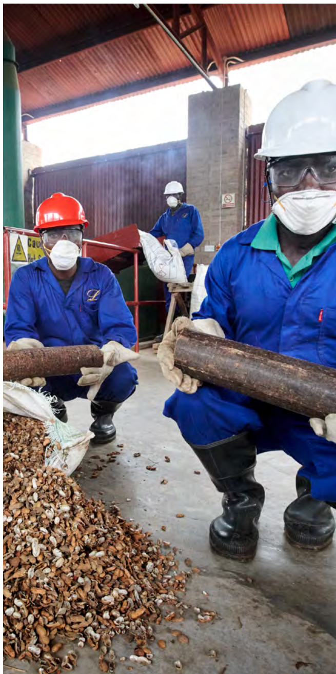
Workers at our local supplier's facility in Malawi holding briquettes made out of groundnut shells and sawdust used as fuel for tobacco curing
