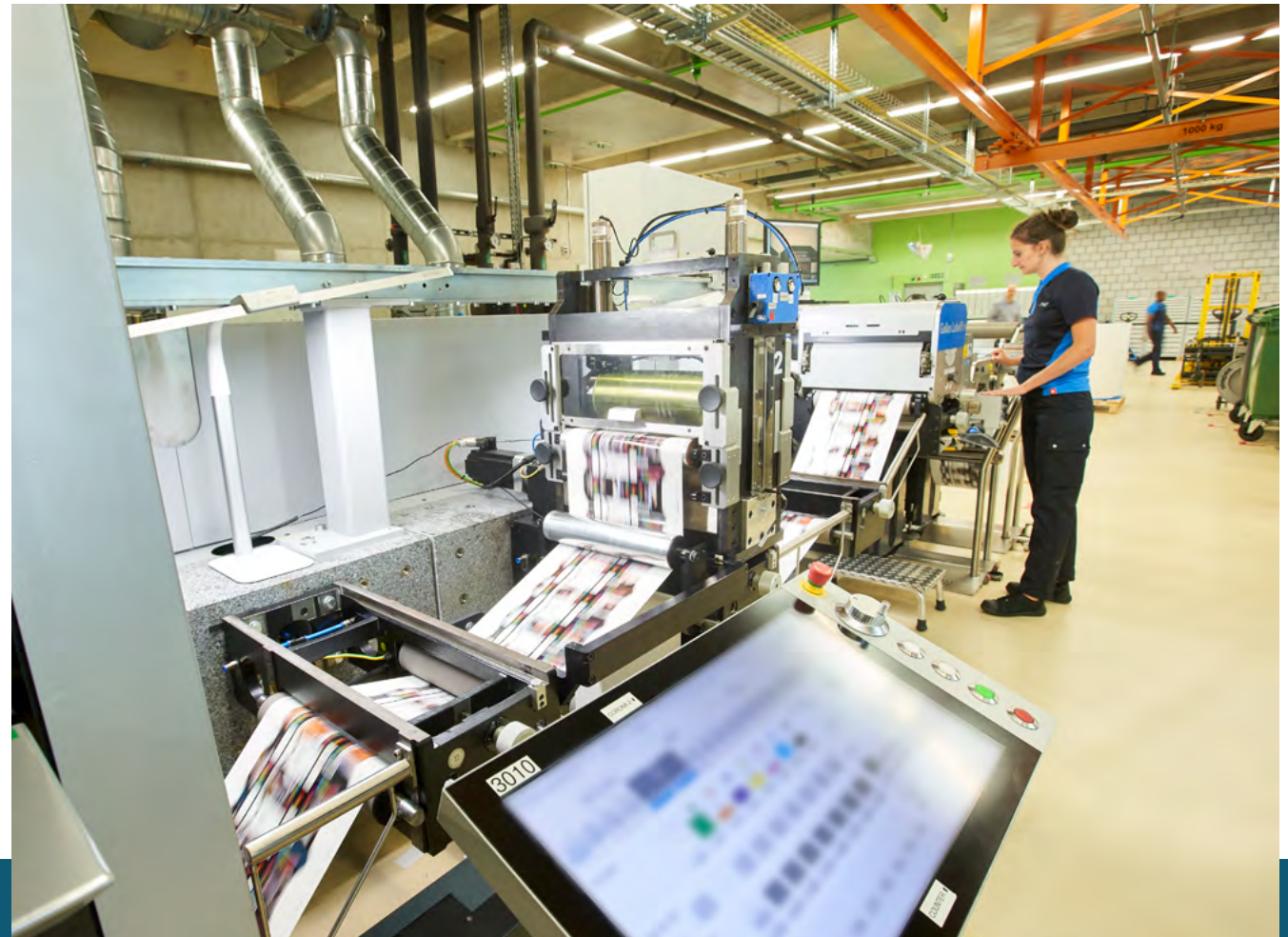
An employee operating the digital printer for packaging material in PMI's manufacturing facility in Neuchâtel, Switzerland
