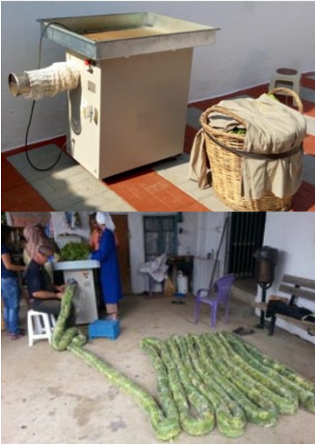
Vento machine used to fill string nets with tobacco for sun curing.
